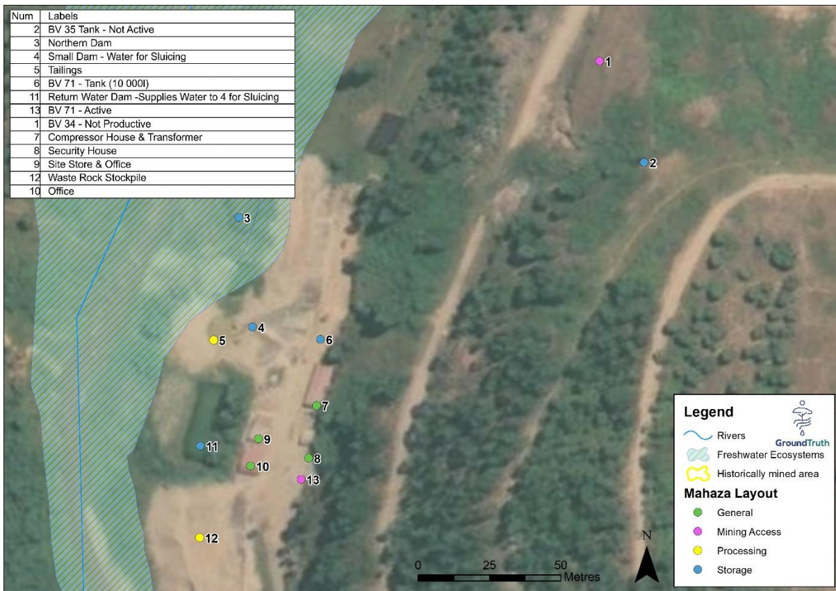
Figure 3-6 Layout of Mahaza Mine (satellite site)
