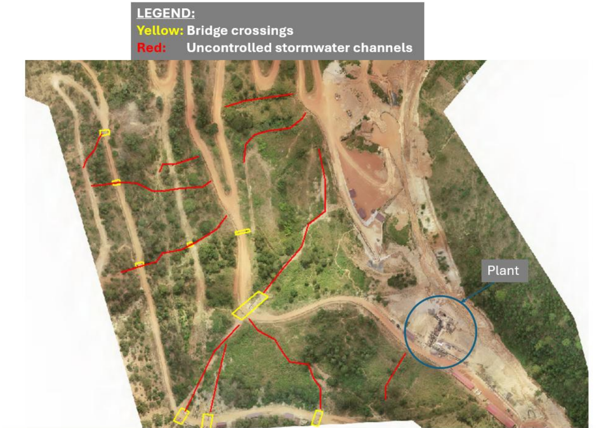
Figure 1-2: Bridge crossings (yellow circle) and eroded stormwater paths (red lines), LiDAR image 2022. Critical infrastructure in the area (mine entrances (tunnel/shafts), processing plant equipment, and worker facilities situated near valley bottoms) are unprotected. The current culvert/bridges is undersized, which has led to overtopping and wash-away in past storms. A new minimum bridge span and vertical clearance will be recommended in this report.
