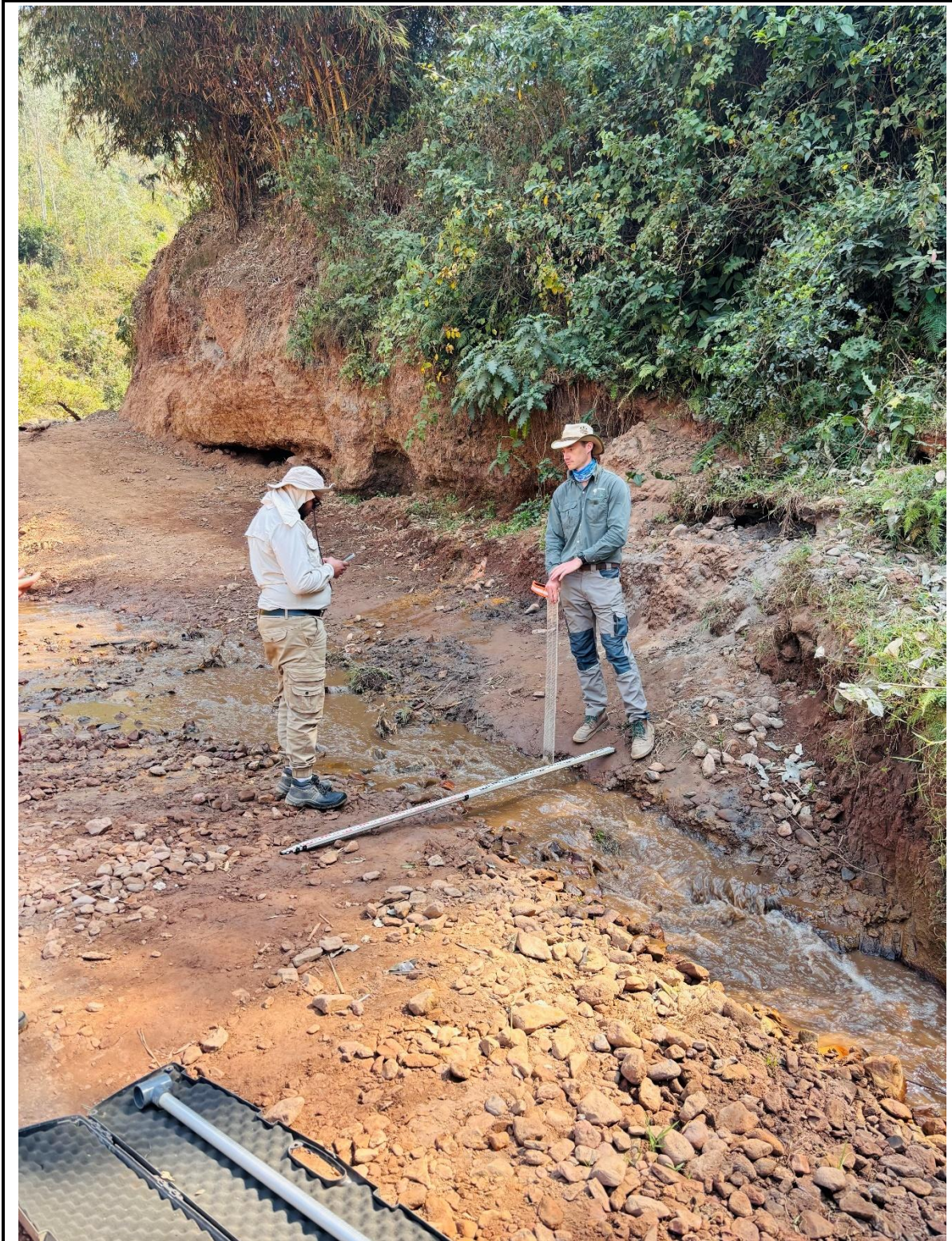
Photograph showing team members measuring waters depths and velocities in the watercourse.
