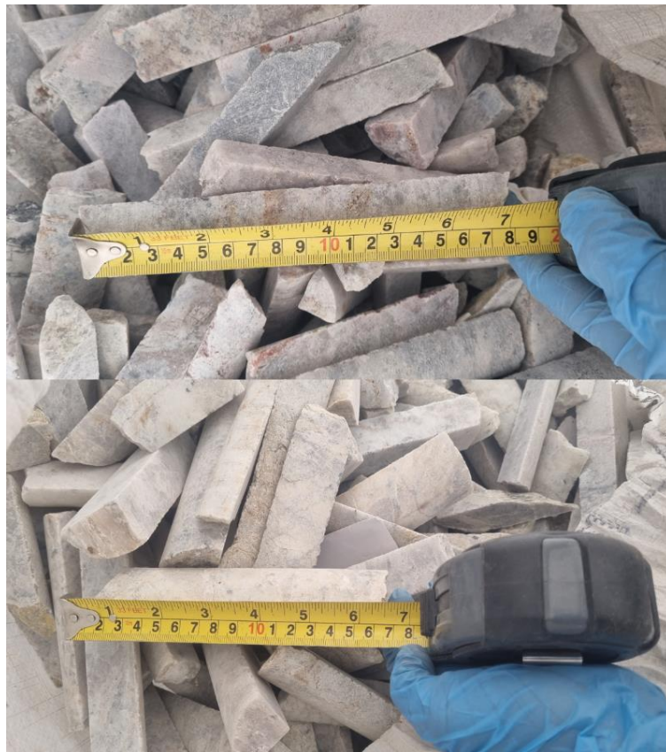
Figure 3 - Scaled images of received quarter core
